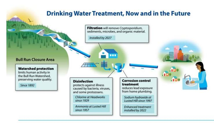
The Portland Water Bureau is in the process of two major treatment improvements for Bull Run drinking water. While the Bull Run is a well-protected watershed requiring minimal treatment for drinking water, enhanced treatment will better meet current regulations, provide increased public health protection from lead in household plumbing and *Cryptosporidium*, provide more consistent water quality, and serve as an investment against future regulations.
